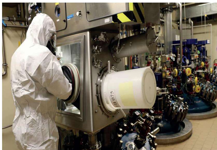
Reactor filling using glove box with alpha beta port
