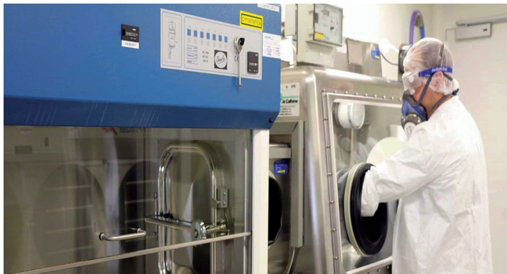
Working in a HAPI class 5 small scale production laboratory in a glove box connected to a laminar flow hood
